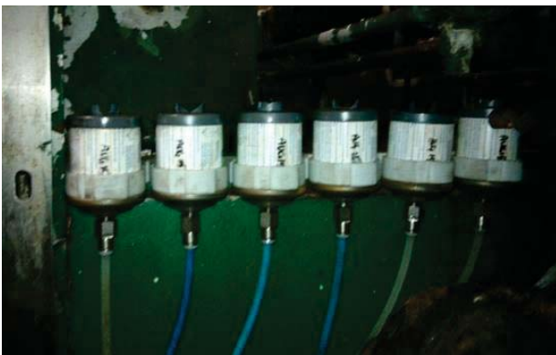
GreaseMax oil units, mounted in brackets, P/N GF10001
