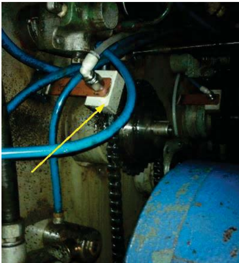
GreaseMax oil units, mounted in brackets, P/N GF10001
