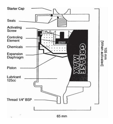
**GREASE MAX** erequires a minimum of approximately 8 hours for a type 1 unit to approximately 40 hours for a type 12 unit to develop sufficient internal pressure to commence discharging lubricant. This period is normally not a problem for well maintained bearings however if lubrication is required in less than the start up period then activate **GREASE MAX** in advance.
